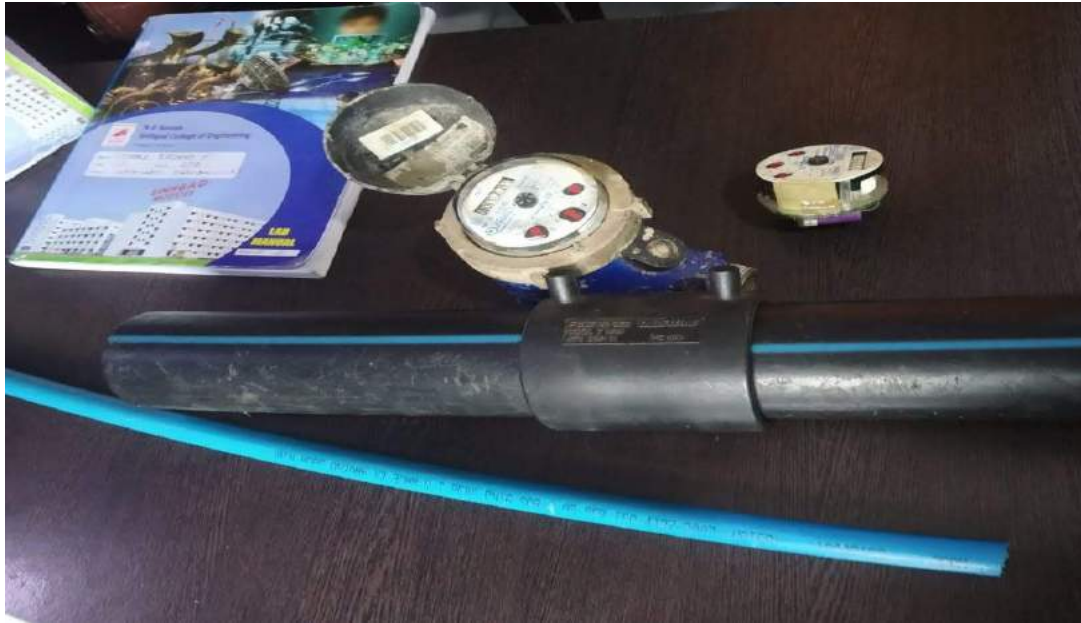
Photo no.1: Illustrates HDPE Pipe
